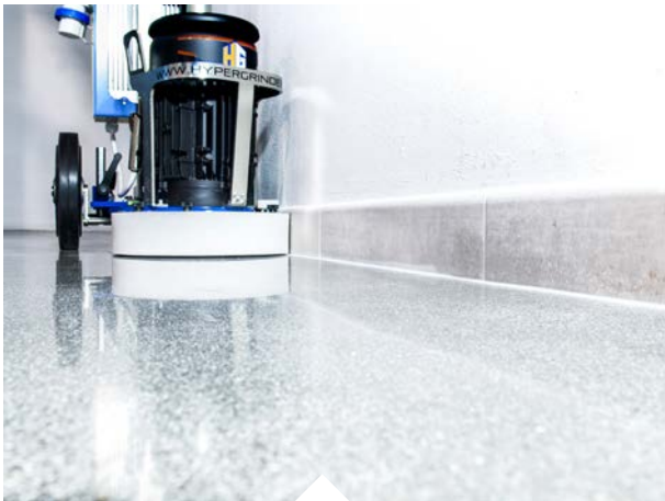
On-board polishing with HCR and GIAGUAR FLEX resinoid disks.
